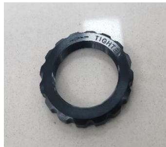
Chainwheel lock nut (Locking torque: 20-24Nm)
