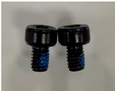
Cylinder head pattern screw M4x6 (Terminal box) (Locking torque: 2.5-3Nm)
