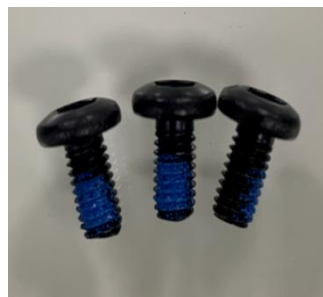
Hexagon socket head screws M4X8 (for cover) (Locking torque: <math>< 1\text{Nm}</math>)
